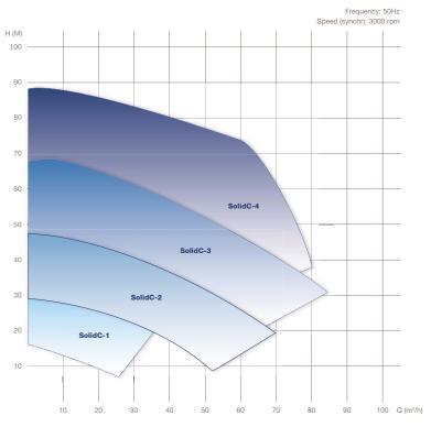
**SolidC performance** SolidC is a reliable, cost-effective centrifugal pump for standard duties up to 85 m<sup>3</sup>/h.
